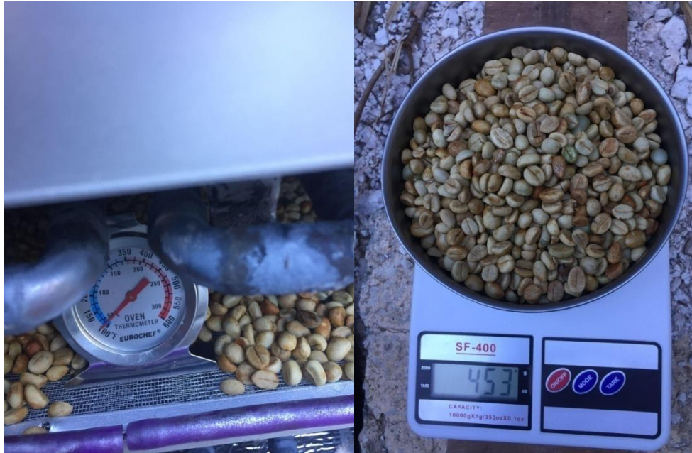
Figure 31. The coffee beans underwent weighing, revealing a reduction in weight from 402 grams to 297 grams. (4:51 PM)
