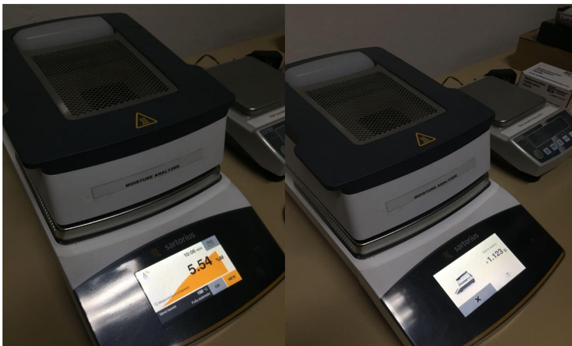
Figure 25. 3rd trial: 1.123 grams = 5.54 %M = 10:06 min
