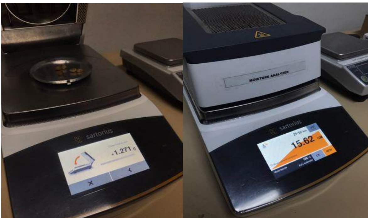
Figure 24. 2nd trial: 1.271 grams = 15.62 % = 21.12 mins (FAILED)
