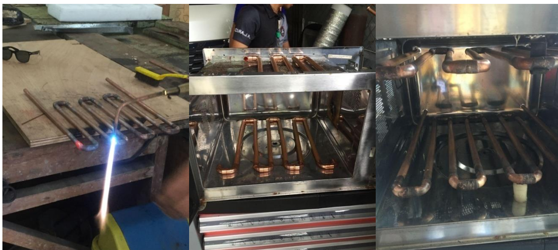
Figure 16. Fabrication of the seven (7) Looped Copper Tubes
